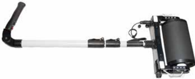
The SSP is a light-weight ground penetrating radar with excellent ergonomic design features. The picture at the right shows how the radar is held when scanning the mine roof
