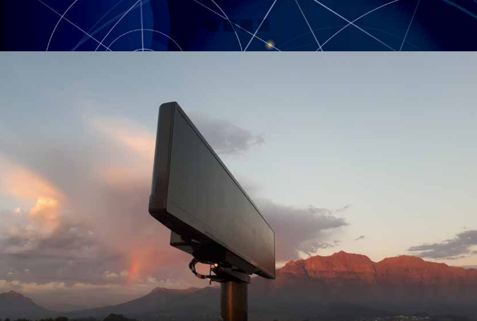
The antenna of the RSR 312 against a backdrop of Stellenbosch mountains. The antenna also houses the transmit and receive electronics
