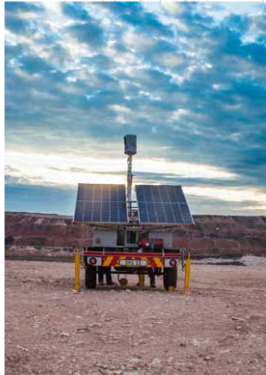
Berm Monitoring System
