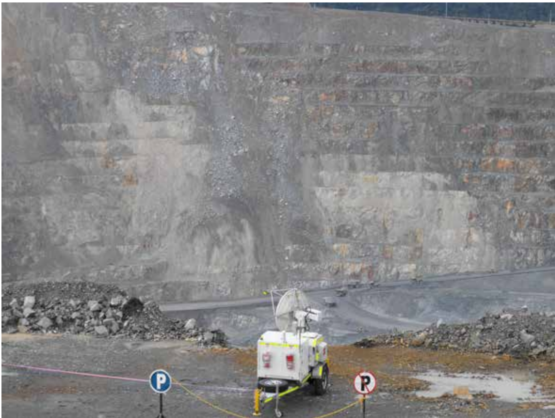
The MSR at the open-pit copper mine at Batu Hijau, Sumbawa Island
