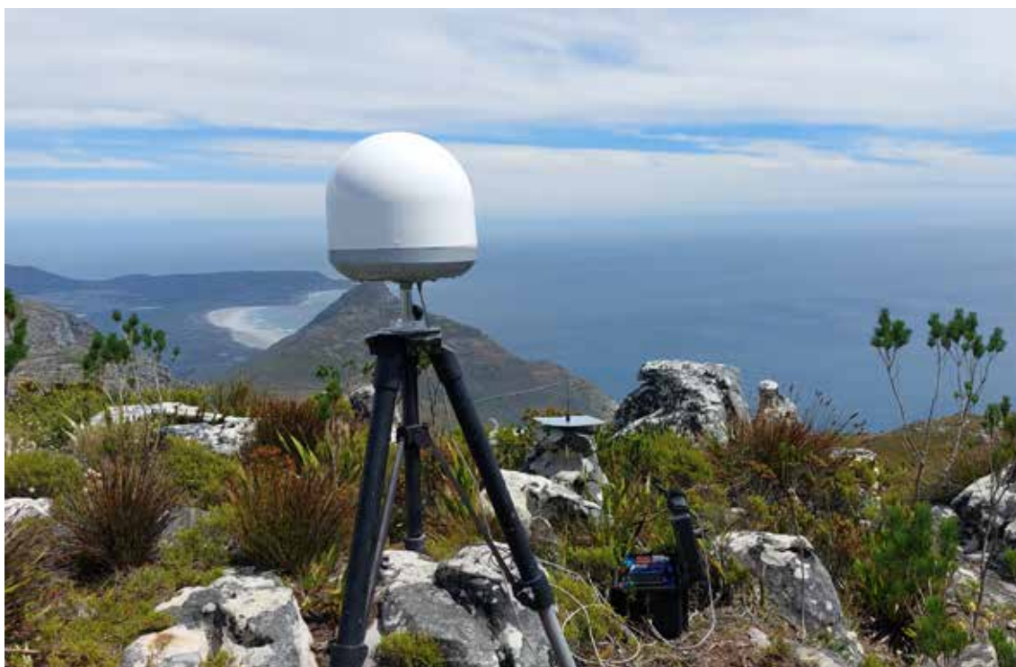
An NRIS intercept receiver can be set up in locations with minimal infrastructure
