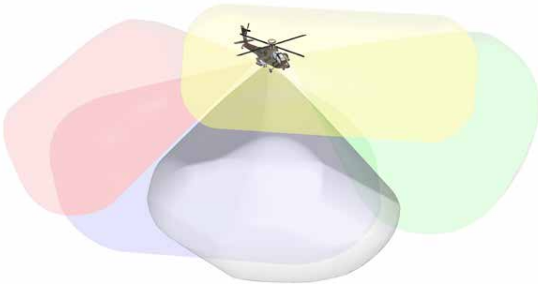
A helicopter is equipped with four sensors covering the four quadrants towards the side and a fifth sensor to cover the ground directly below the helicopter
