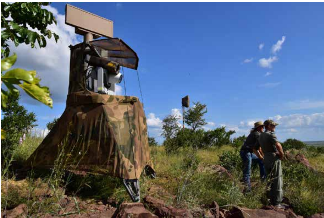
The Meerkat system keeps a 24/7 watch over the rhinos in the Kruger National Park. The RSR 904 radar initiates a response when it detects moving objects.
