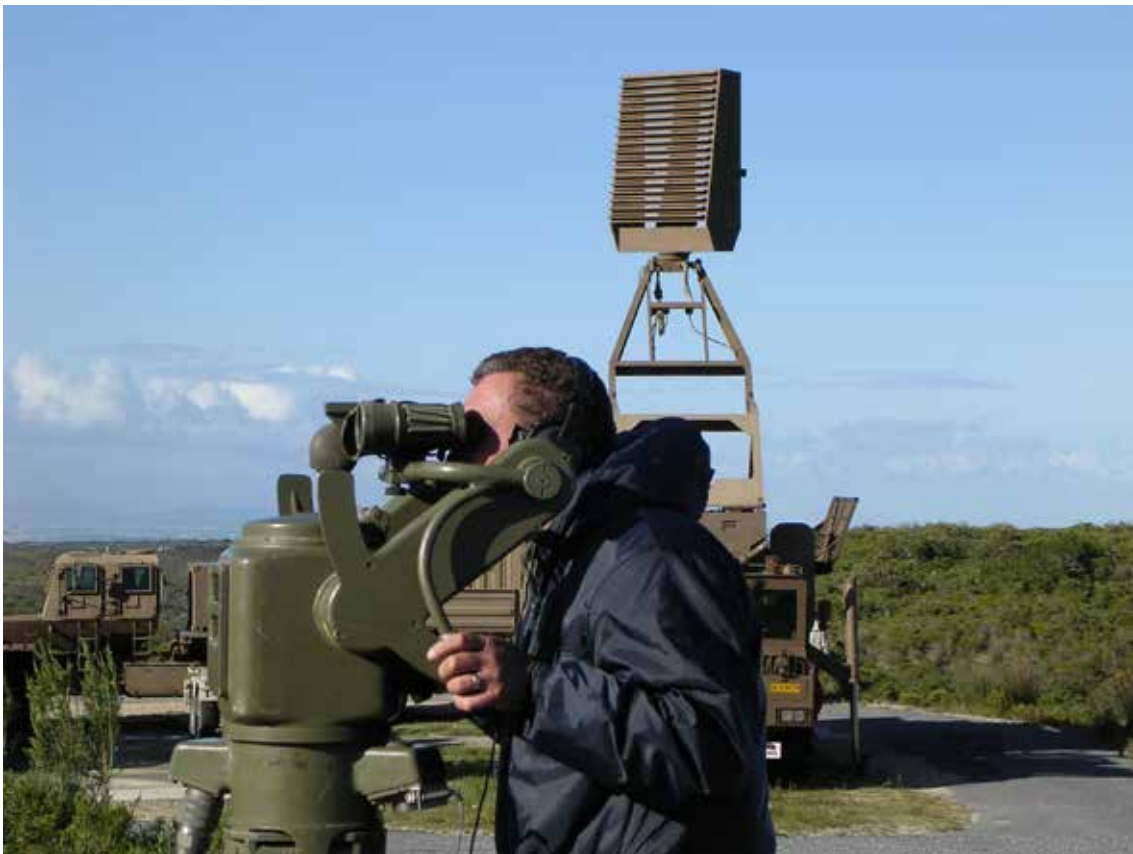
An optical 'Put-er On-er' (South African slang for an optical target designator) in use during the ORT trials
