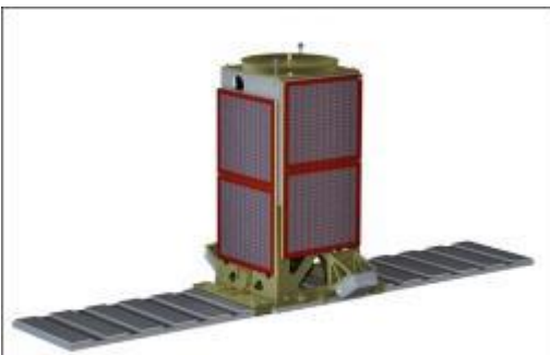
Figure 22: Looking forward, this image shows a CAD rendering of the design for a satellite SAR payload and bus, jointly being developed with a South African micro-satellite manufacturer.
