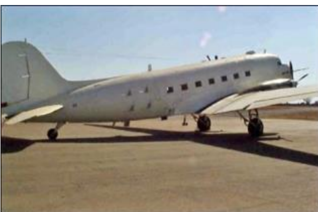
Figure 18: SASAR system installed on a SAAF C-47TP Turbo Dakota. Notice the VHF Antennas protruding from the aircraft skin aft of the rear windows.
