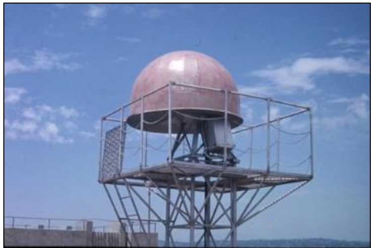
Figure 4: The PUMAR X-band pulse compression surveillance and target acquisition radar (left) with its antenna deployed for testing on the roof of the NIDR building in Pretoria (right).
