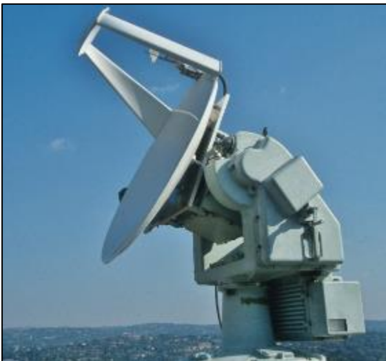
Figure 9: The MECCANO wide band monopulse tracking radar antenna being tested on the rooftop of Building 44 at the CSIR in Pretoria.
