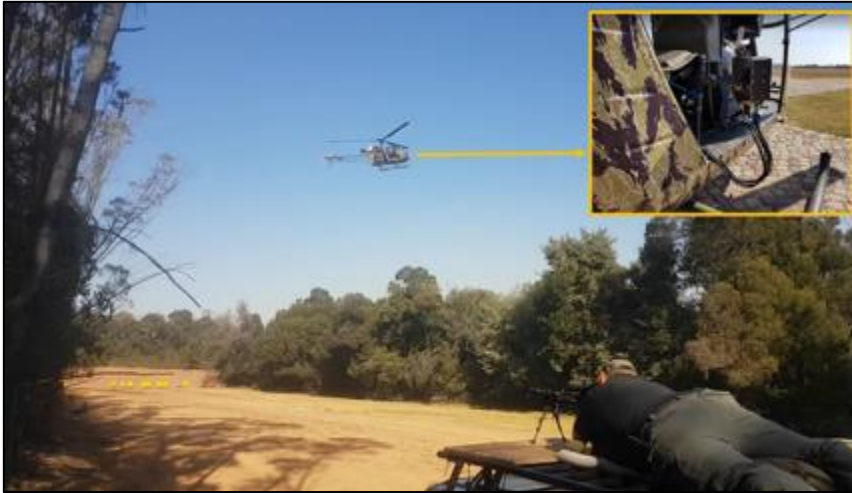
Figure 17: Live bullet firing tests with the hostile fire indicator hardware demonstrator mounted on an Alouette II helicopter.
