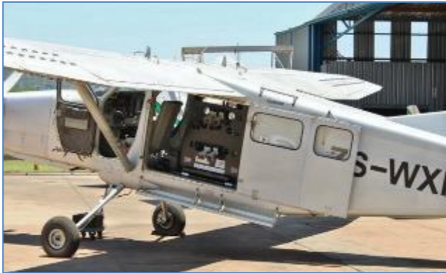
Figure 20: The DSI SAR airborne facility installed in an Atlas Angel aircraft ready for flight tests.
