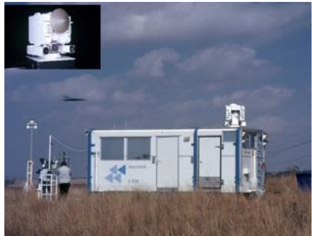
Figure 8: The FYNKYK Ka-Band Monopulse Tracking Radar in its mobile laboratory during field testing against a Mirage F1 fighter aircraft outside Irene, near Pretoria.
