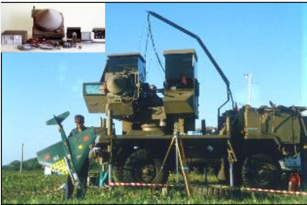
Figure 7: The NIMBUS Ka-band range-only radar, integrated with the technology demonstrator of a 20 mm GBADS Gunnery System also developed at the NIDR, during field testing at the St Lucia test range.
