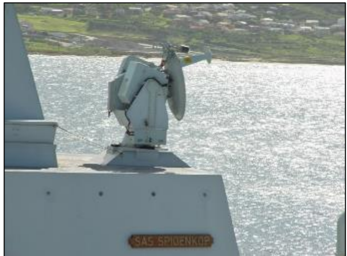
Figure 10: The Reutech Radar Systems RTS 6400 Optronic Radar Tracker installed on the SA Navy frigate SAS Spioenkop.
