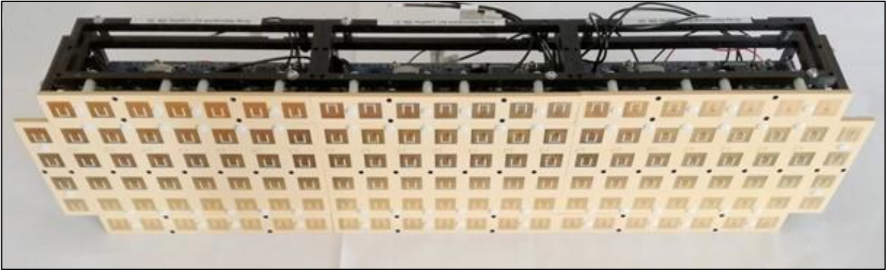
Figure 15: An integrated C-band phased array antenna consisting of three 7 channel AESA T/R panels.
