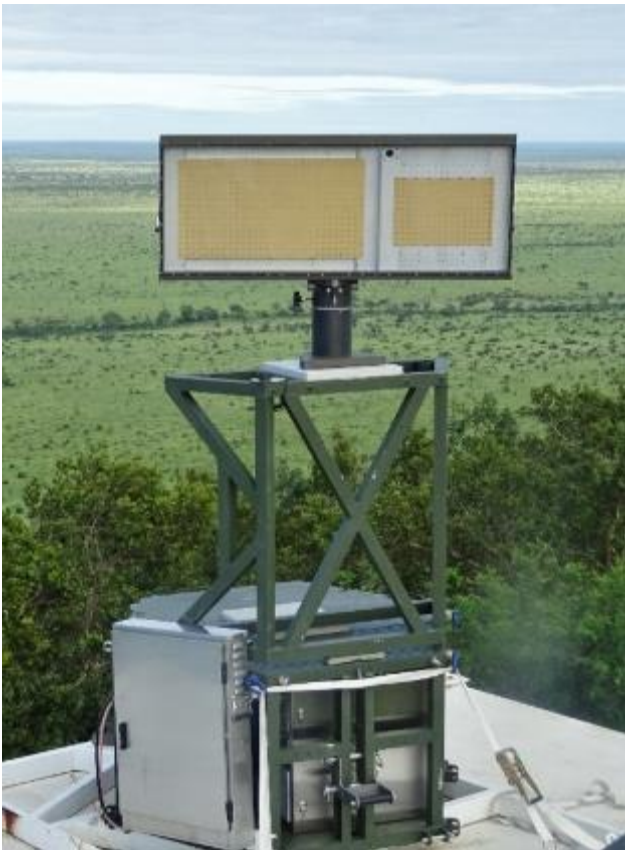
Figure 13: The GSCR with its separate transmit and receive AESA antennas deployed in the KNP for its first set of field trials in February 2021.
